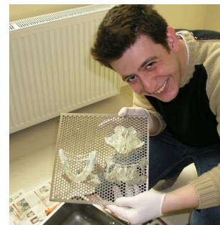
3D-printed mandible from a tomography scan
